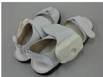
Wearable triaxial ground reaction force sensors
